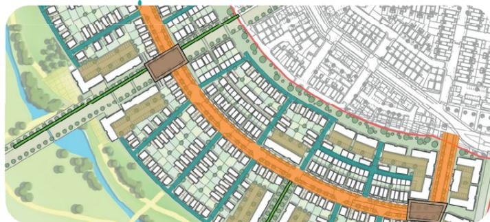
Extending the swale network to include primary and secondary streets reduces embodied carbon from the stormwater network, whilst also increasing the provision of 'blue/green networks'. This highlights the general principle of reducing materials used, in place of nature-based solutions that help deliver holistic benefits, including climate resilience.
