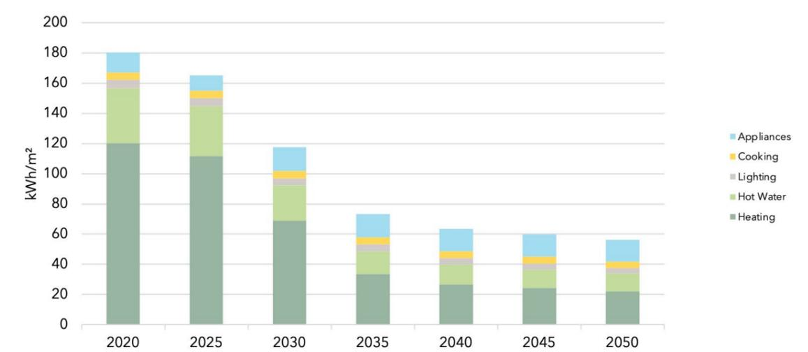
**Figure 17:** Resultant existing dwelling energy use intensity (kWh/m<sup>2</sup>/yr)
