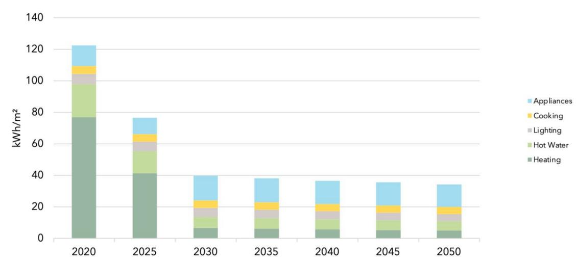
**Figure 16:** Resultant new dwelling energy use intensity (kWh/m<sup>2</sup>/yr)
